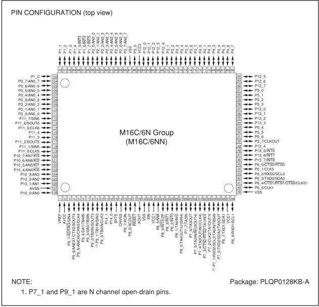
Figure 1.4 Pin Configuration (Top View) (2)
